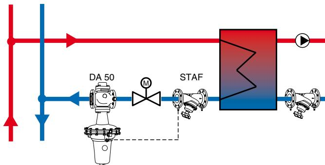
The controller has to be installed in the return pipe, downstream the consumer (DA 50) or in the inlet pipe, upstream the consumer (DAF 50).
