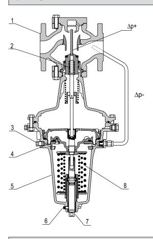
Installation in bypass pipe. The controller consists of a valve (1) and a diaphragm actuator (5). Valve is protected against overload with a safety spring (2).
