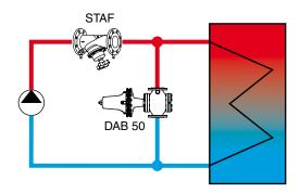
Install the controller in bypass pipe. The direction of flow is shown by the arrow on the valve body. It is recommended to install the controller in horizontal pipeline with actuator body below. Installation of a strainer upstream of the controller is recommended.
