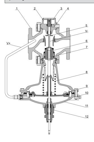
The controller consists of a valve (1), a diaphragm actuator (11) and an adapter (12) for the connection of an electromotor actuator for temperature control.
