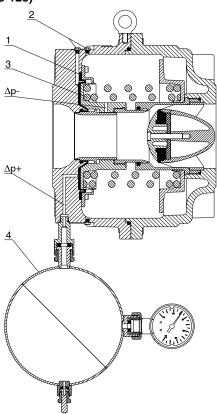
Pressure from inlet acts through internal impulse pipe (P-) to the outlet side of the diaphragm (1) and together with spring force (3) opens the valve.
